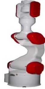
Figure 1. Mitsubishi PA10-6CE robotic manipulator [14]
