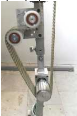
Fig. 4: Belt adjustment mechanism
