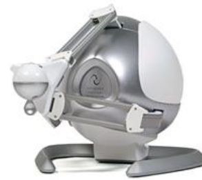
Figure12. Novint Falcon haptic interface Table 2. Properties of Falcon haptic interface
