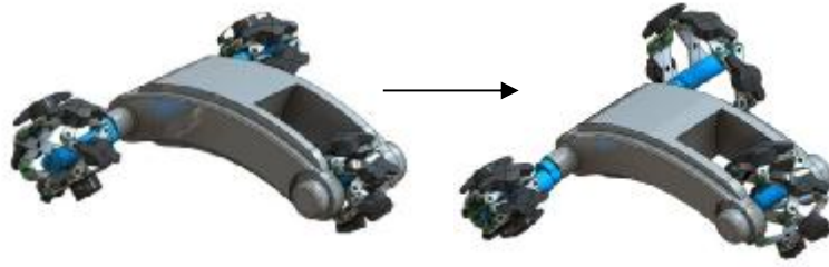
Fig. 3. The complete mobile robot structure with adaptable wheel geometry
