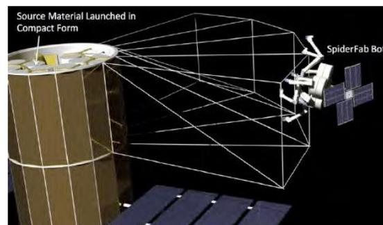
Figure 2. SpiderFab fabricates a support structure onto satellite [18].
