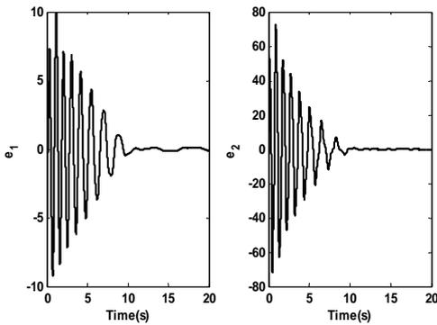
Fig. 6: Time series of synchronization errors with LQR control.
