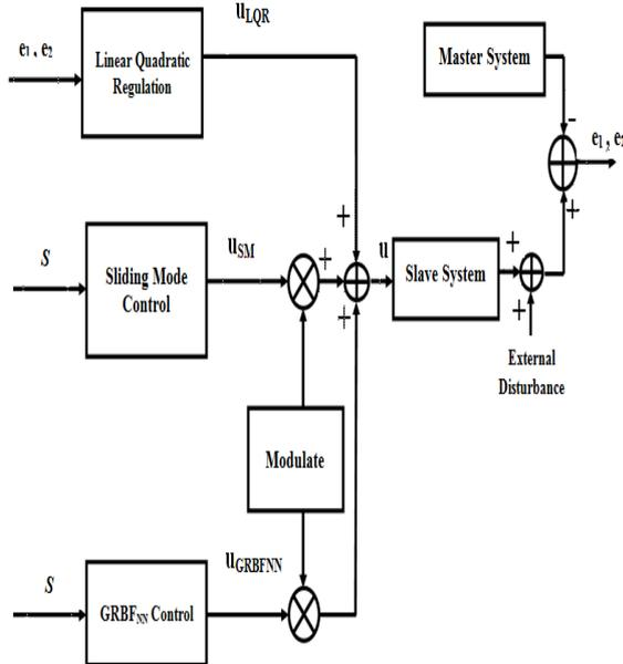
Fig. 3: oscillator Structure of hybrid control to synchronize of chaotic Duffing system.
