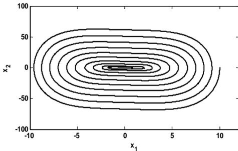
Fig. 2: Phase plane trajectory of a chaotic Duffing oscillator system.
