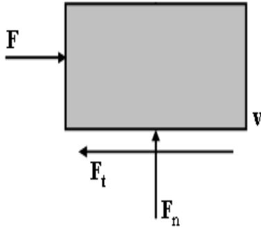
Fig. 3: Free body diagram for a moving object on a surface.
