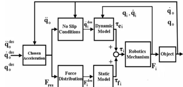
Fig. 5: Structure of the control system.
