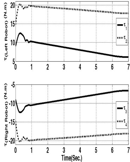
Fig. 15: Time history of manipulators generalized driving forces when the model parameters differ from the actual one.
