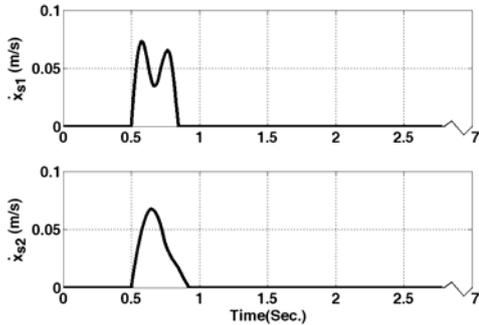
Fig. 14: Sliding velocity when the model parameters differ from the actual one.
