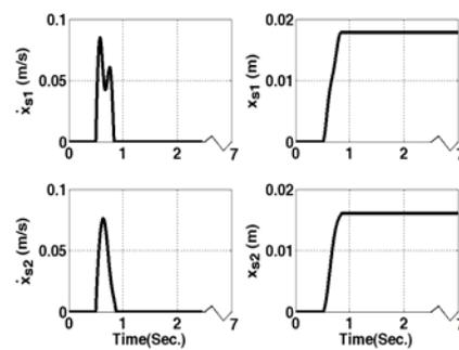
Fig. 10: End-effectors movement on the object surfaces and slippage velocity of the end-effectors.
