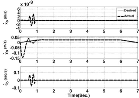
Fig. 13: Object velocity tracking when the model parameters differ from the actual one.
