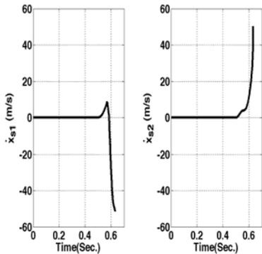
Fig. 12: Slippage velocity of the end-effectors using conventional approach without modification.
