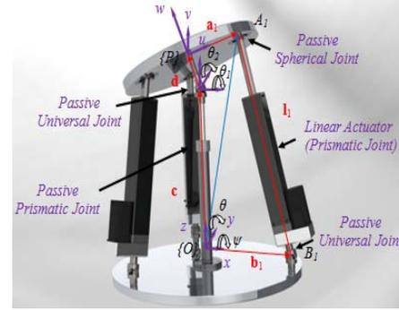
Figure 1: Tricept structure and geometric model.
