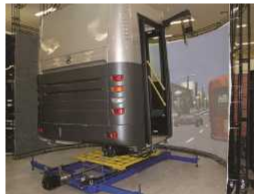
Fig. 1: Urban bus driving simulator built at K. N. Toosi University of Technology.
