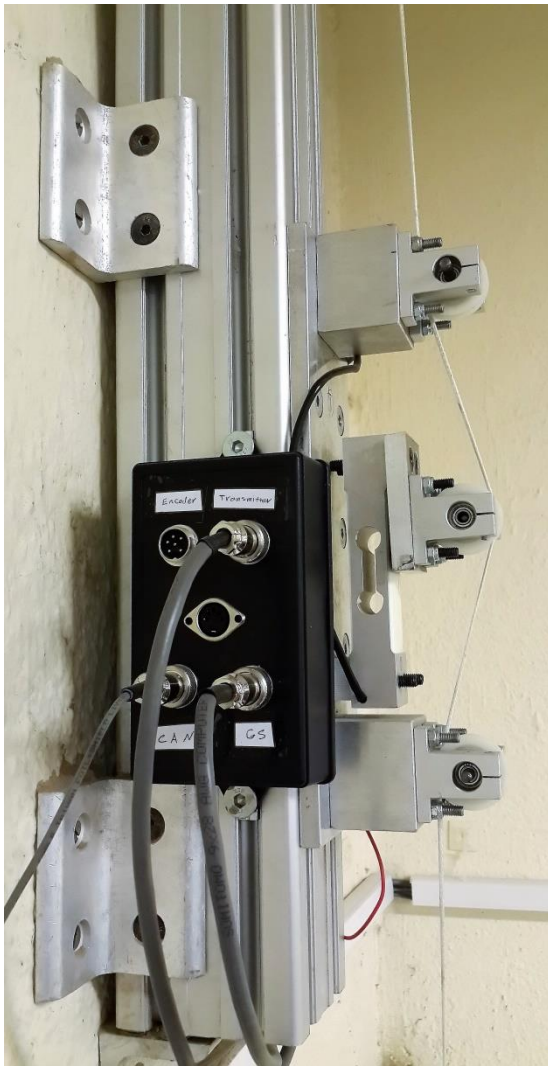
Figure 6. Force sensor system designed to measure cable force
