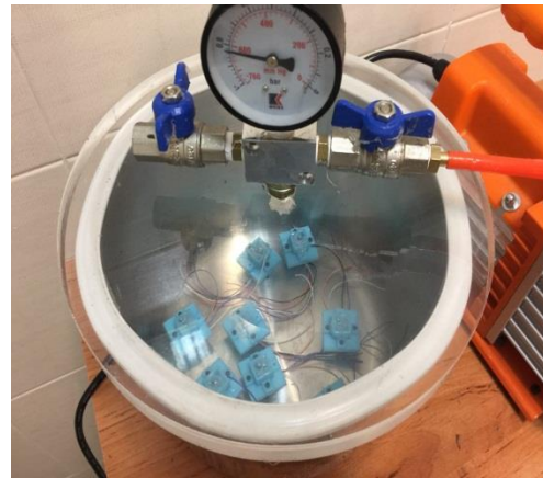
Fig. 8. The vacuum chamber used for degassing the silicon.
