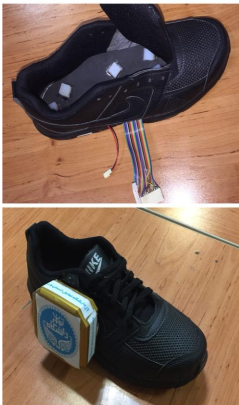
Fig. 12. Final prototype of ShrewdShoe. Top picture shows the insole and connectors and in the bottom picture lateral attachment of the hardware case can be seen.
