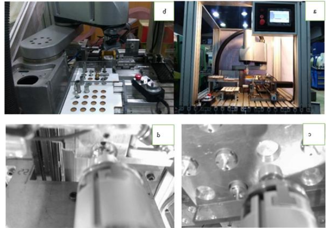
Figure 12: a. Malek Ashtar University (4-dof) Scara robot designed and manufacture for tiny- fine parts assembling b-. Scara robot with Stereo_ IBVS (C922 Logitech PRO camera) mounted on the end effector
