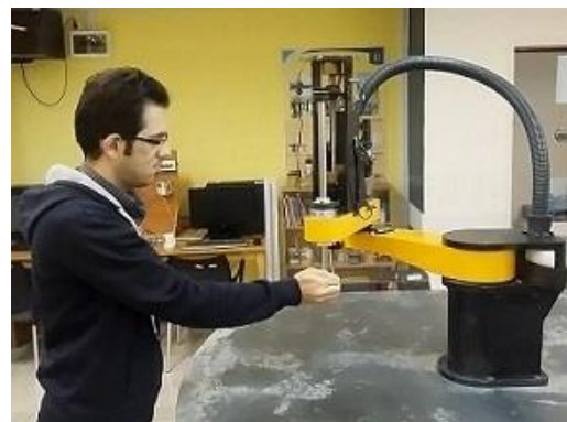
Figure 1. The FUM SCARA robot during teaching by demonstration
